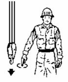
**LOWER**. With arm extended downward, moving hand in small horizontal circles.
