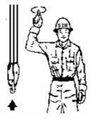
**HOIST**. With forearm vertical, forefinger pointing up, moving hand in small horizontal circles.
