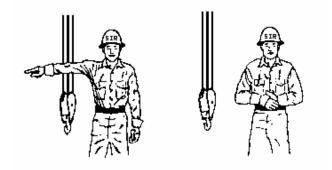
**SWING.** Arm extended, point with finger in direction of swing of boom.
